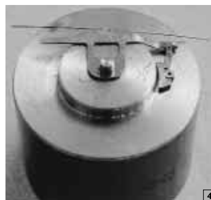
Top: Using a simple tool to emboss the rivets.
