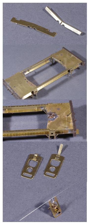
This image shows the slider with the brake shoe. This is folded and laminated up as shown.
