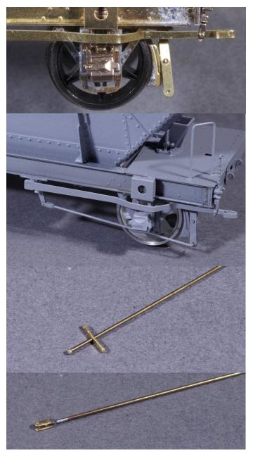
Fit the axlebox sliders to the underframe. The easiest way to do this is to fit one end of the spring and then the other. Centralise the axlebox and gently flex the spring until you can slip the axlebox between the horns.
