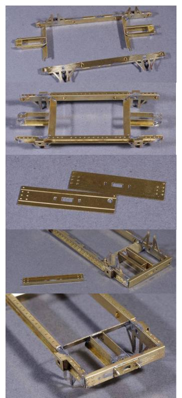
Add some washers to the top side of the coupler mount, solder in place and then drill/tap M1 for coupler mounting.
