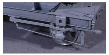
Drop the hopper in place. It should contact the solebars on all four side shoes (Also in the pockets, but this will not be
