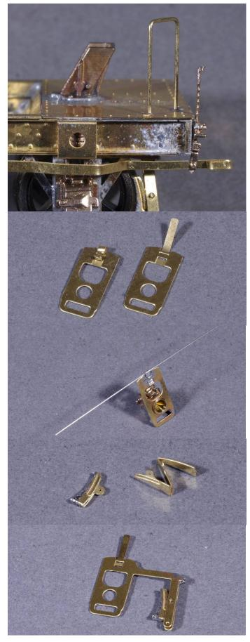
Note that the hanger needs to be inclined outwards at the lowest point. The brake shoe should be gently twisted so that it remains vertical.
