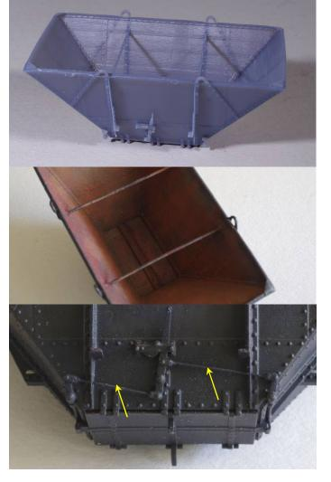
Fit upper door surface into the hopper using CA glue.
