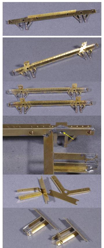
Locate lugs on underframe inner parts into slots in solebars and solder up.
